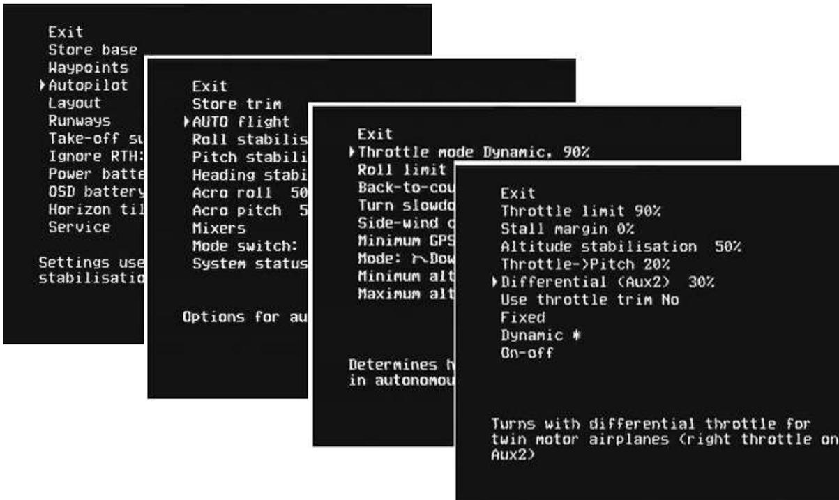
In this option you may disable differential throttle (default settings) by selecting **OFF**, or enable it by selecting proper differential throttle mixer value (percentage). In most cases this value should be equal to transmitter's **rudder->differential throttle** mixer value.
